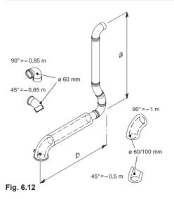
Each additional elbow reduces the overall acceptable length of the flue system as follows:
